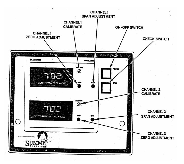
Figure 5: IR-702 Front Panel
