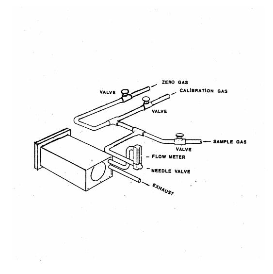
Figure 4: Typical Gas Handling System
